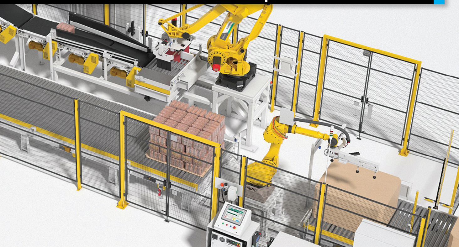
Brenton's latest bag palletizing solution for pet manufacturers replaces gantry solutions with an automated sheet placing robot. Image courtesy of Brenton Engineering.
