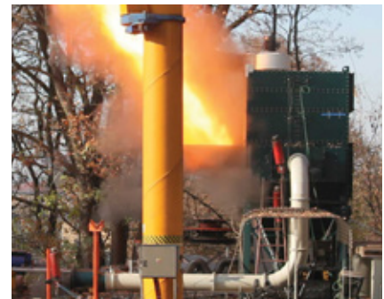
The flame is almost immediately diverted away from the dust collector to a safe area.
