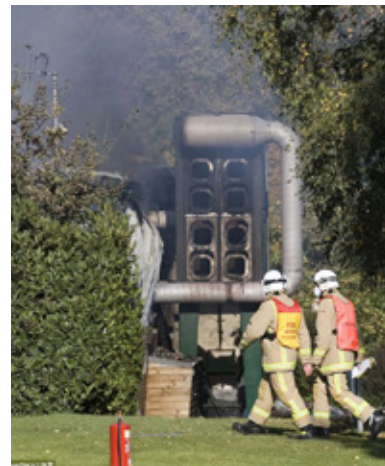
Toner dust explosion in the UK.
