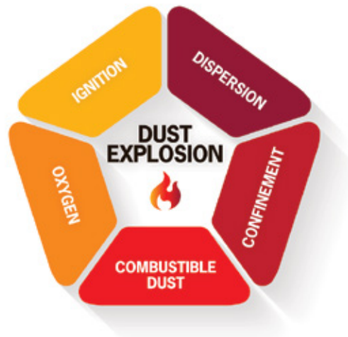
Figure 1: Dust explosion pentagon shows the elements that must be present for a combustible dust explosion to occur.
