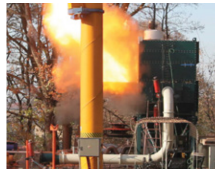
About 5 milliseconds later, the dust ignites and the vent opens.
