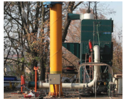
At the startup of a staged explosion, explosive dust is injected into the dust collector to create a flammable cloud.
