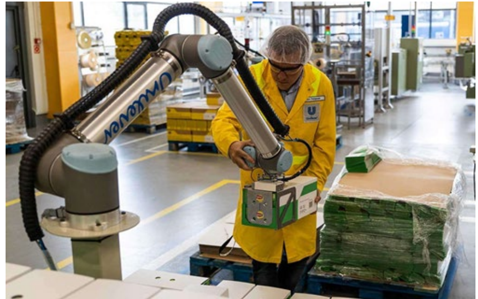
Unilever has deployed UR10 cobots to handle palletizing tasks at the company’s Katowice, Poland facility. Source: Universal Robots
