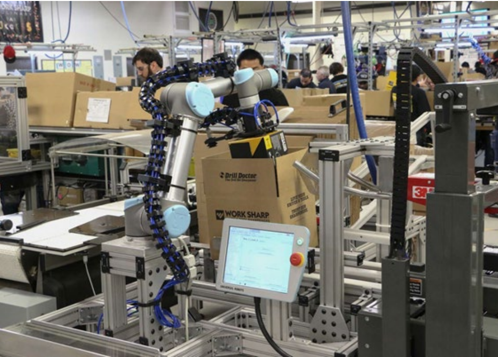
Darex deployed a UR5 cobot from Universal Robots to handle packaging and palletizing tasks. Source: Universal Robots
