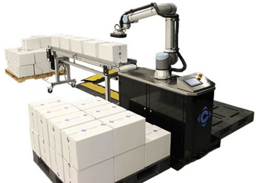
The Cross Palletron 300 Application Kit comes with a 7th axis, which increases the cobot's work envelope compared to 6-axis systems. Source: Universal Robots
